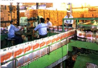
Closed supervision and automatic filling machines ensure quality and quantity in lubricant tins.
