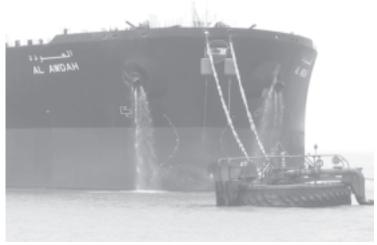
Single Point Mooring off Vadinar coast in the Gulf of Kutch, the discharge point for Very Large Crude Carriers bringing in imported crude oil for onward movement to Koyali, Mathura and Panipat refineries by pipelines.
