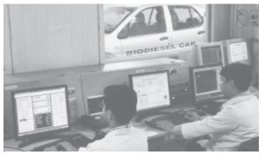
IndianOil scientists conducting test runs on various blends of Bio-diesel with diesel in the climatic chamber of the R&D Centre as part of commercialisation efforts in alternative fuels.
